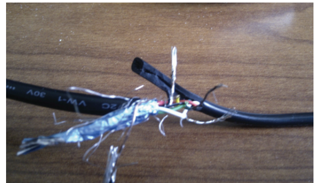
Figure 6: The Crafted USB Cable for Phone-to-Phone Attacks.
